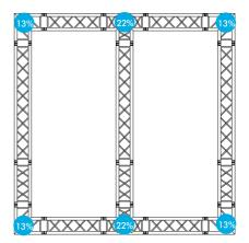
Assuming that each truss node represents a support, the approximate support reactions are given here as a percentage of the total uniformly distributed load of a square construction with a central truss.
