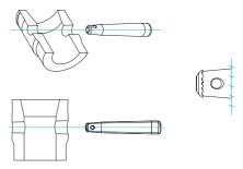
Deformation of the conical pins.
