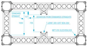
Figure : H30V-C017 with MPT sleeve blocks
