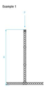
to match the given situation. The buckling length sk of a tower is calculated by multiplying the buckling factor  $\beta$  by the tower height A.
