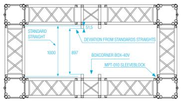
Figure: BOX-40V with MPT sleeve block
