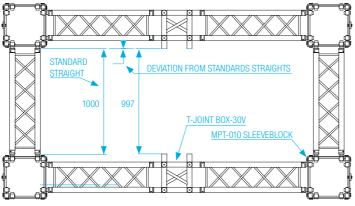
Figure: BOX-30V with MPT sleeve blocks
