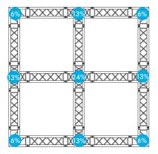
distributed load for a construction with X30D trusses of c. 1026 kg. This means support loads of:
